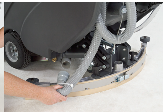
For a full-functioning extractor, move the hose to the vacuum shoe inlet and raise the squeegee.
